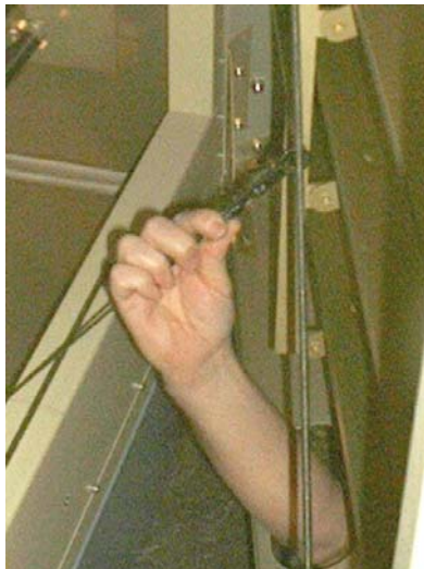
Fig. 5-4. Reaching through the access port to disconnect cable
