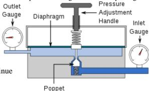
Figure 5: Regulator diagram created by Mintrick.
