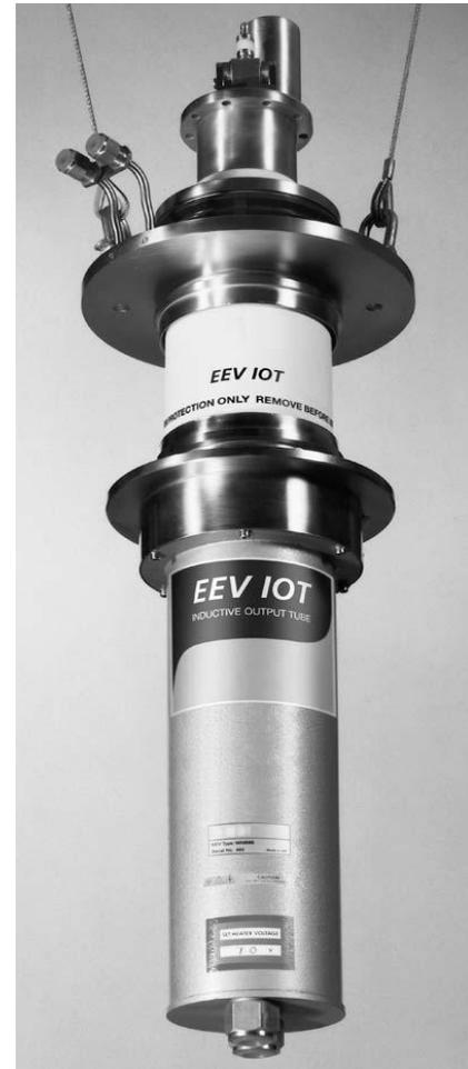
Figure 2: Inductive output tube.
