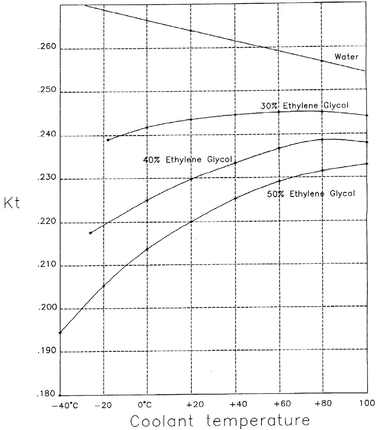
**Fig. 10 Kt for Ethylene-Glycol/Water Mixtures vs. Temperature**
